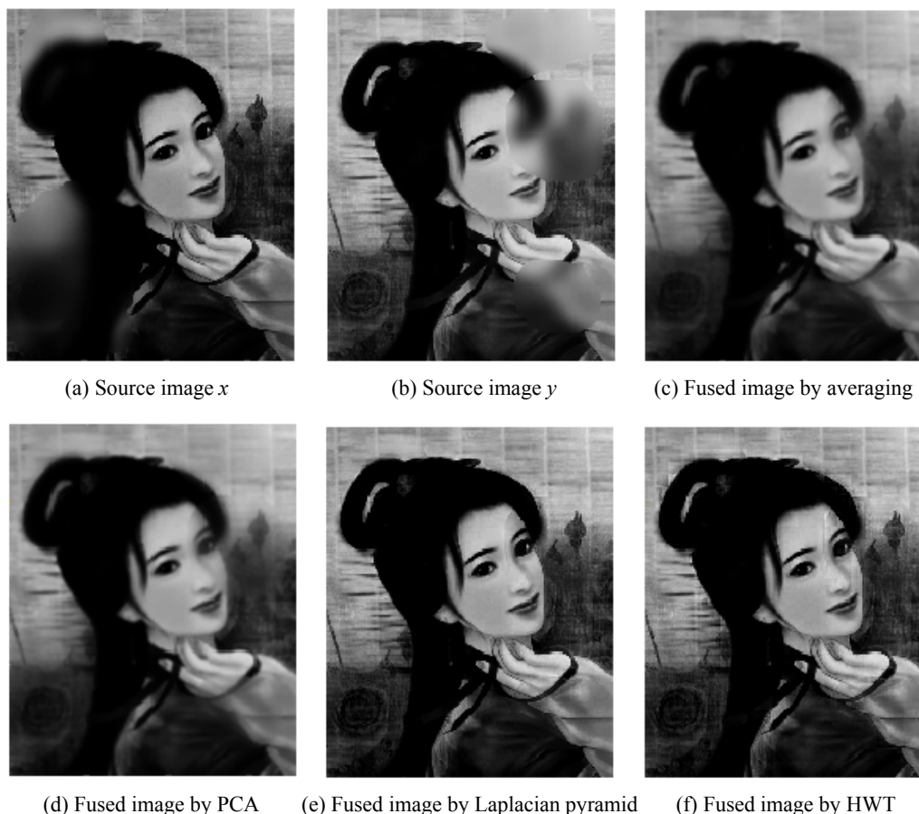
Fig. 3 Fusion of blurred and Gaussian noise augmented images
