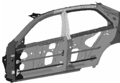
Fig. 1 Side structure of the selected car
