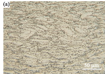
(a) Optical micrograph of FeAl
