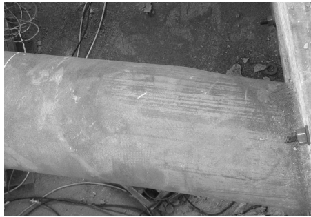
(b) Lüders slip lines in part of tube
