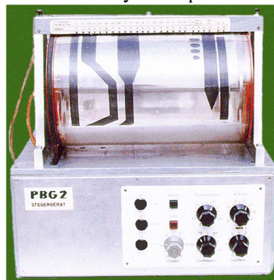
Fig. 5. Device for playing back spectrograms, TU Dresden 1973 (Historic acoustic-phonetic collection of the TU Dresden).
