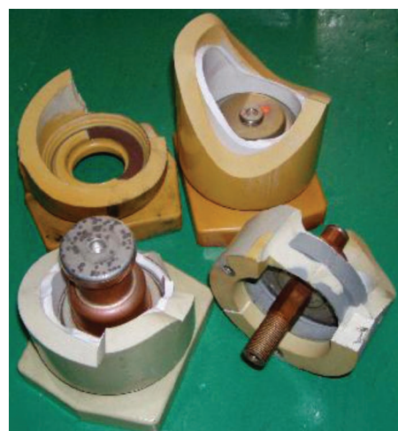
Figure 2. Test samples molded from conventional epoxy compounds.
