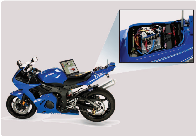
FIGURE 2. The modified 2004 Yamaha YZF-R6 motorcycle. The factory ECU was removed from under the seat and replaced with the National Instruments CompactRIO embedded control system in the tail of the motorcycle.
