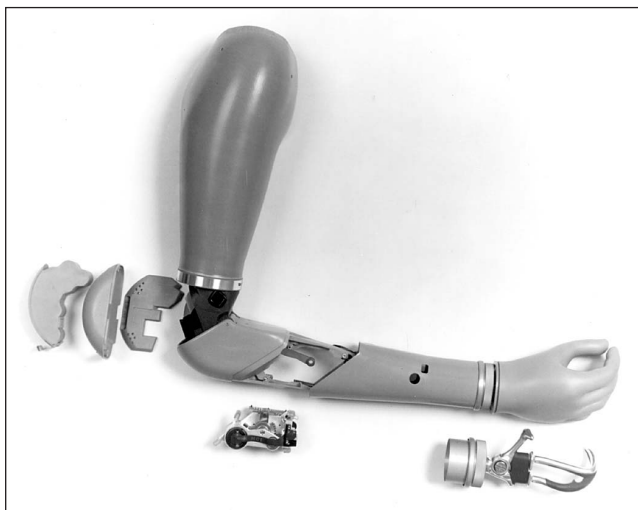
The original Utah Artificial Arm was developed in 1980. The internal control circuits are housed in smooth molded plastic covers that are light, strong, and cosmetic.
