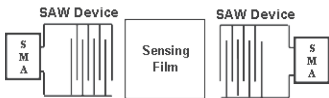
Fig. 5 Schematic layout of SAW resonator sensor for relative humidity monitoring
