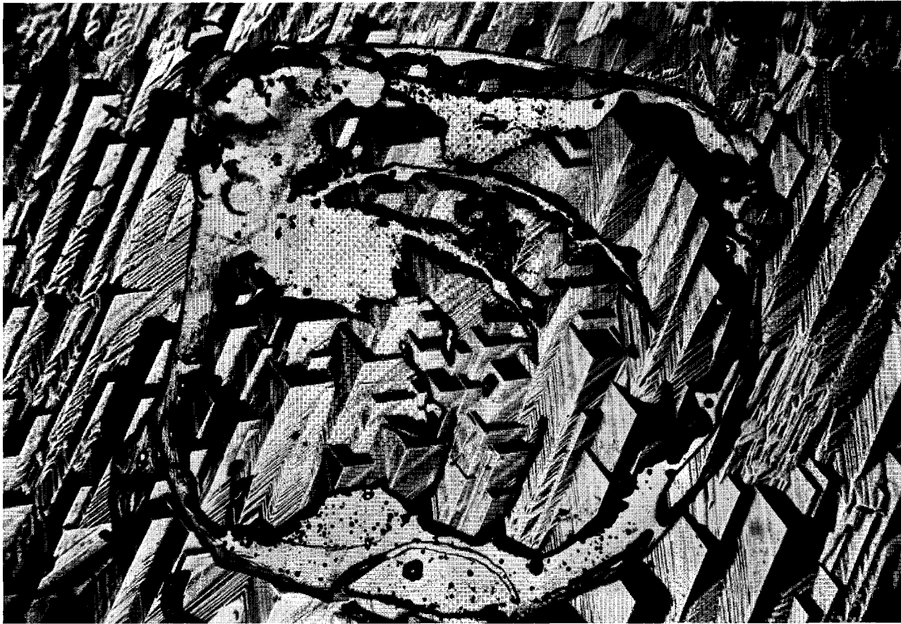
Figure 9 Chemical impurities on substrate surface impeding nucleation and subsequent crystal growth. (65X)
