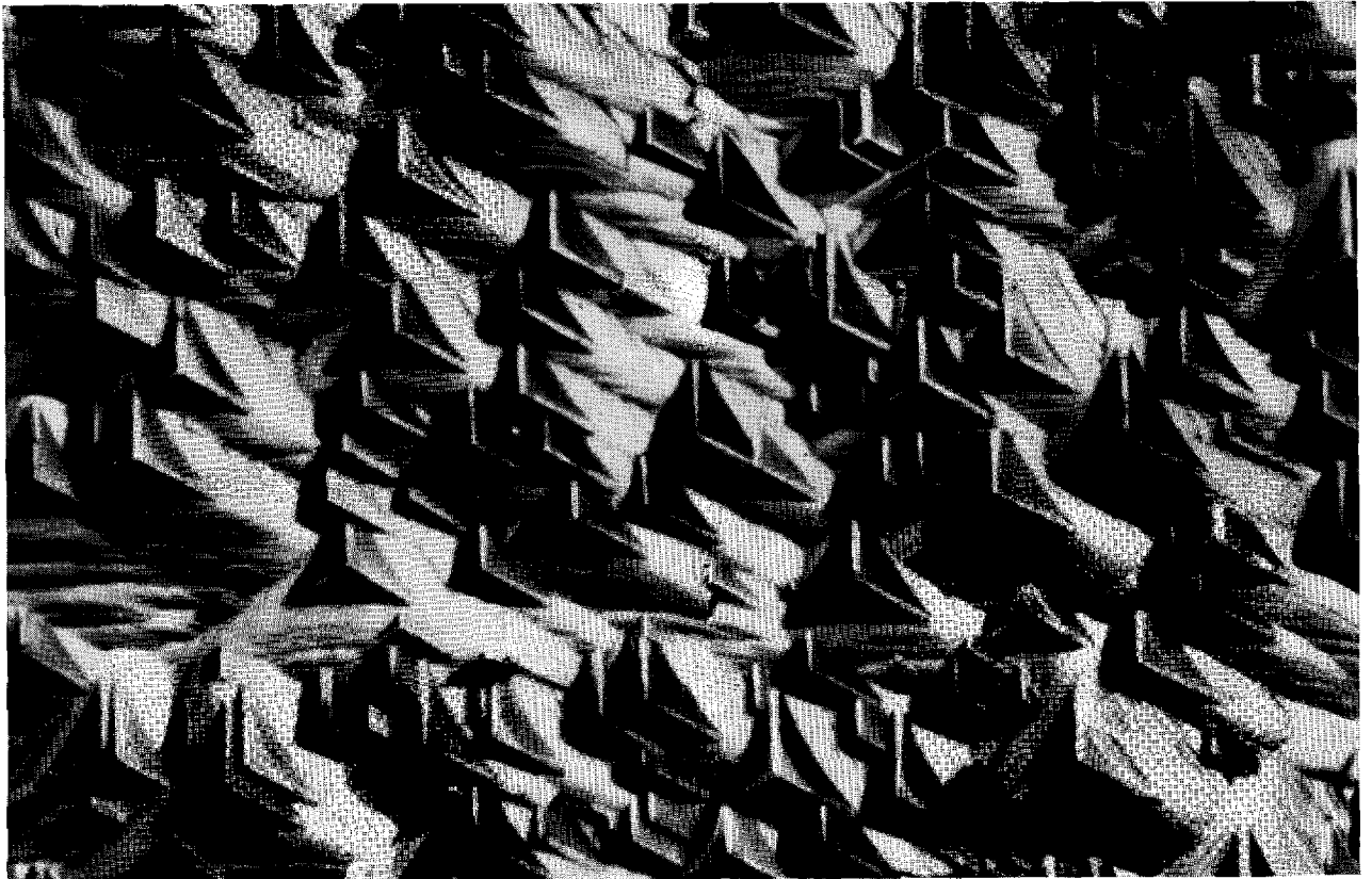
Figure 5a Typical epitaxial growth on the (111) silicon substrate. (200X)
