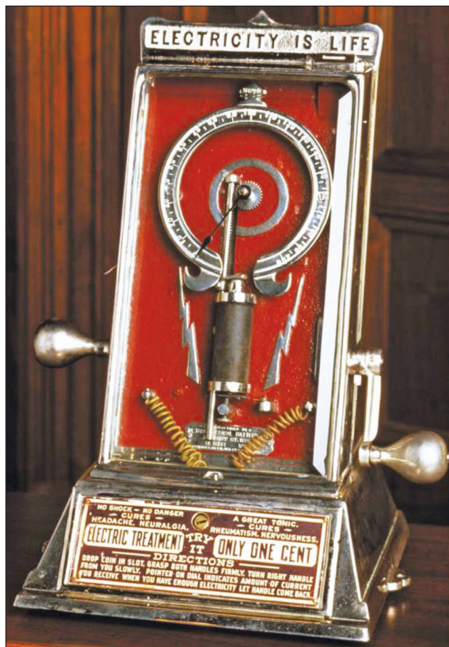
Fig. 3. Arcade shocker for treating headache, neuralgia, and nervousness ca. 1900. Customers grabbed the handles to receive therapy.
