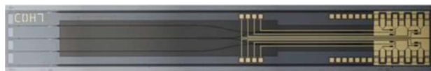
Fig. 13. Photograph of a monolithically integrated InP dual-port coherent receiver for 100-Gb/s PDM-QPSK. The chip size is 8 \times 1.2 \text{ mm}^2 [241]. ©2011 OSA.
