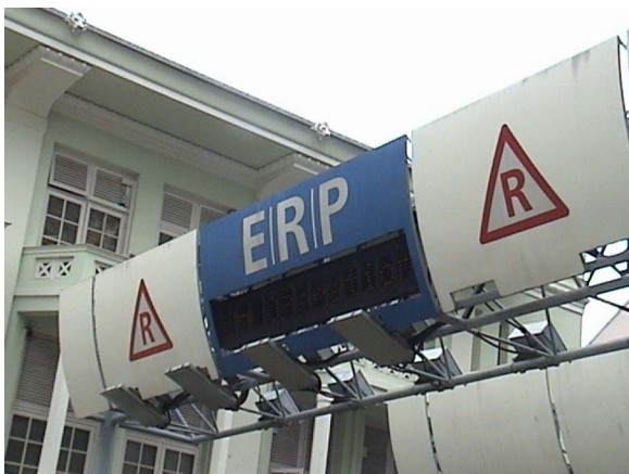
Fig. 5. Singapore's Electronic Road Pricing (ERP) system. The ERP uses a dedicated short-range radio communication system to deduct ERP charges from CashCards. These are inserted in the in-vehicle units of vehicles before each journey. Each time vehicles pass through a gantry when the system is in operation, the ERP charges are automatically deducted. Courtesy of Katina Michael 2003.
