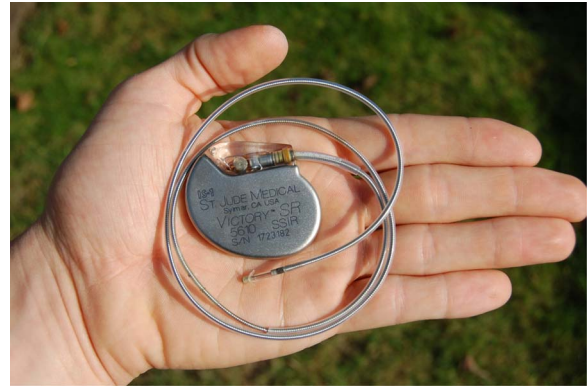
Fig. 18. An artificial pacemaker from St. Jude Medical (St. Paul, MN), with electrode 2007. Courtesy of Steven Fruitsmaak.
