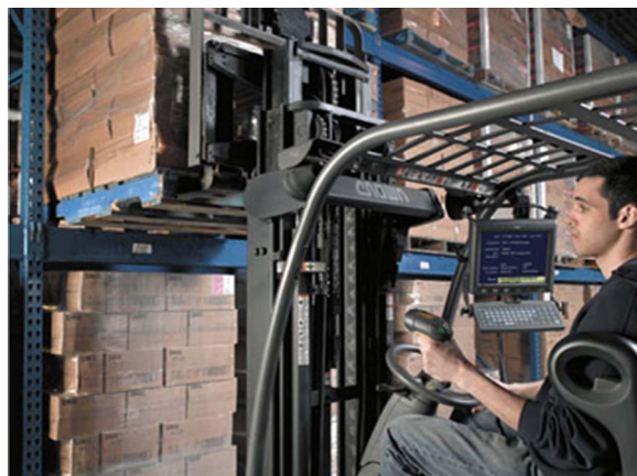
Fig. 8. Barcodes printed on individual packaged items on pallets. Order information is shown on the forklift's on-board laptop and the driver scans items that are being prepared for shipping using a handheld gun to update inventory records wirelessly. Courtesy AirData Pty Ltd, Motorola Premier Business Partner, 2009.
