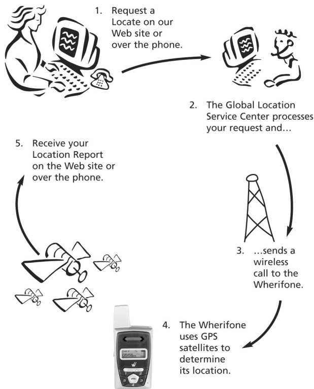
Fig. 9. A five step overview of how the Wherify location-based service works. The information retrieved by this service included a breadcrumb of each location (in table and map form), a list of time and date stamps, latitude and longitude coordinates, nearest street address, and location type. Courtesy of Wherify Wireless Location Services, 2009.
