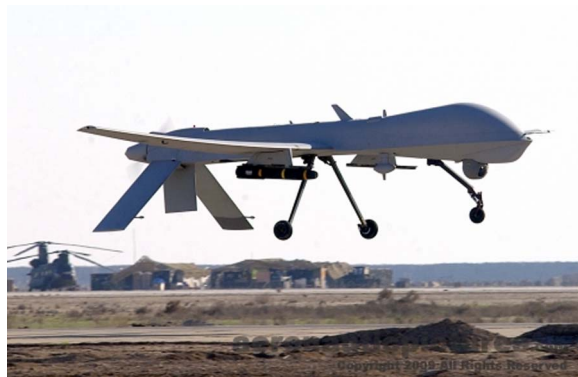
Fig. 14. Predator Drone aircraft: this plane comes in the armed and reconnaissance versions and the models are known as RQ-1 and MQ-1.
