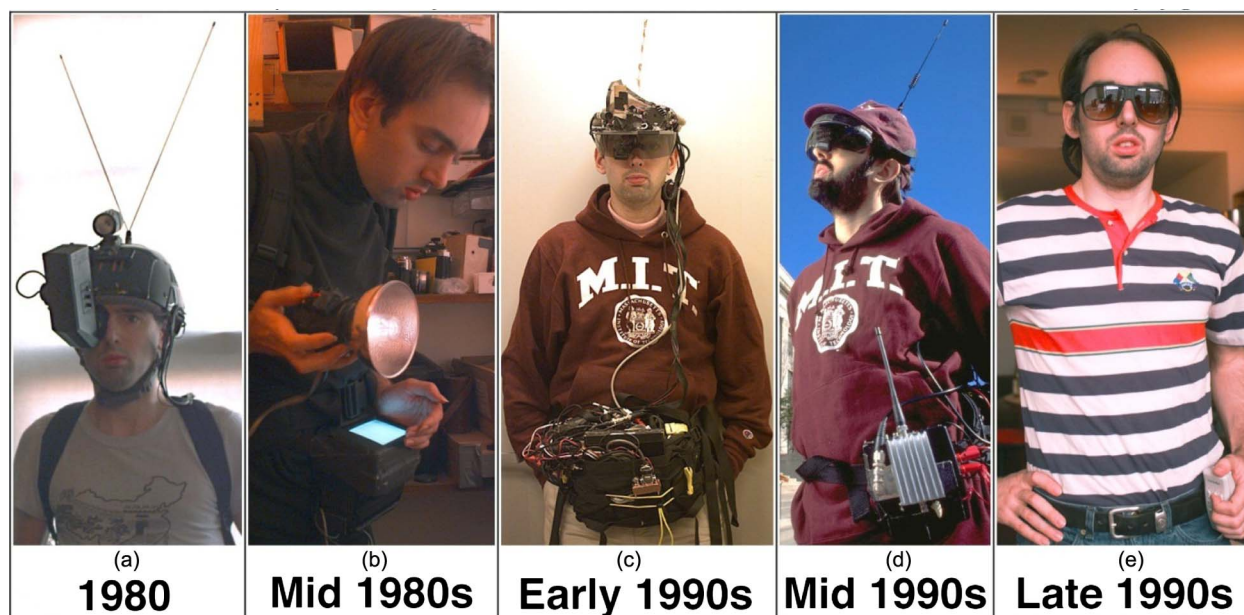
Fig. 12. Self-portraits of Mann with wearable computing kit from the 1980s to the 1990s. Prof. Mann started working on his WearComp invention as far back as his high school days in the 1970s. Courtesy of Steve Mann.
