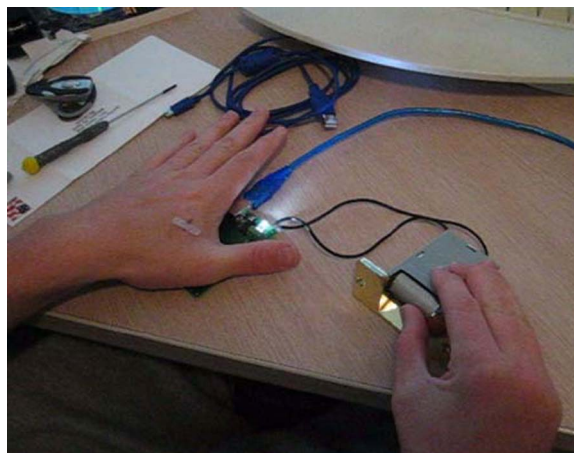
Fig. 20. Amal Graafstra demonstrating an RFID-operated door latch application he developed. Over the RFID tag site on his left hand is a single steri-strip that remained after implantation for a few days. His right hand is holding the door latch.
