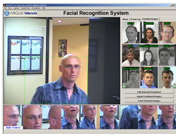
Fig. 4. A facial recognition system developed by Argus Solutions in Australia. Increasingly facial recognition systems are being used in surveillance and usually based on video technology. Digital images captured from video or still photographs are compared with other precaptured images. Courtesy of Argus Solutions 2009.
