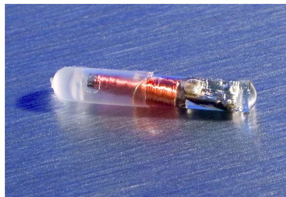
Fig. 19. The VeriChip microchip, the first microchip implant to be cleared by the U.S. Food and Drug Administration (FDA) for humans, is a passive microchip that contains a 16-digit number, which can be used to retrieve critical medical information on a patient from a secure online database. The company that owns the VeriChip technology is developing a microscopic glucose sensor to put on the end of the chip to eliminate a diabetic’s need to draw blood to get a blood glucose reading. Courtesy of PositiveID Corporation.
