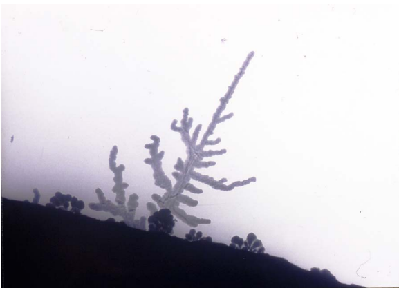
Fig. 7. Lithium dendrites being formed on electrodeposition of lithium, from [18].
