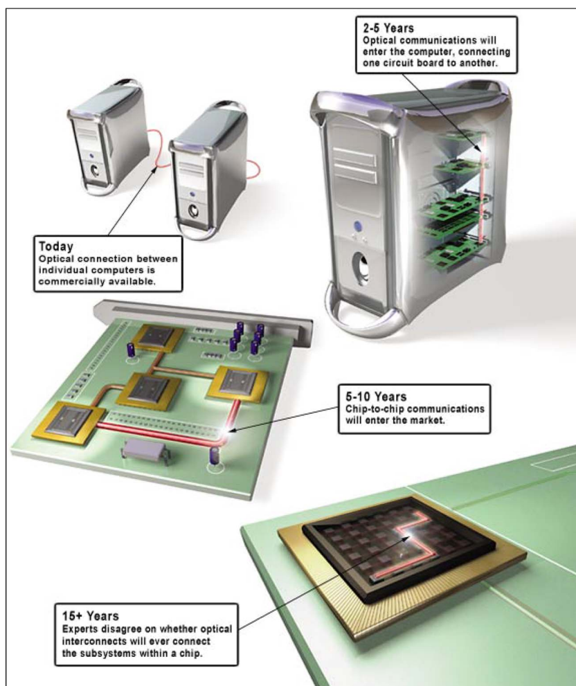
Fig. 5. Schematic illustration of optical link evolution in future computer systems discussed in the 2002 IEEE SPECTRUM article “Linking with light” [51].
