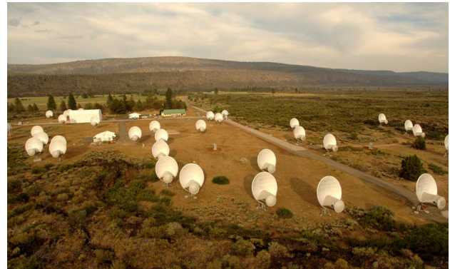
Fig. 2. Aerial view of the Allen Telescope array, now consisting of 42 antennas each 6.1 m in diameter, at the Hat Creek Radio Astronomy Observatory in northern California. The array can be used simultaneously for SETI observations and more traditional radio astronomy projects. Credit: G. Seth Shostak.
