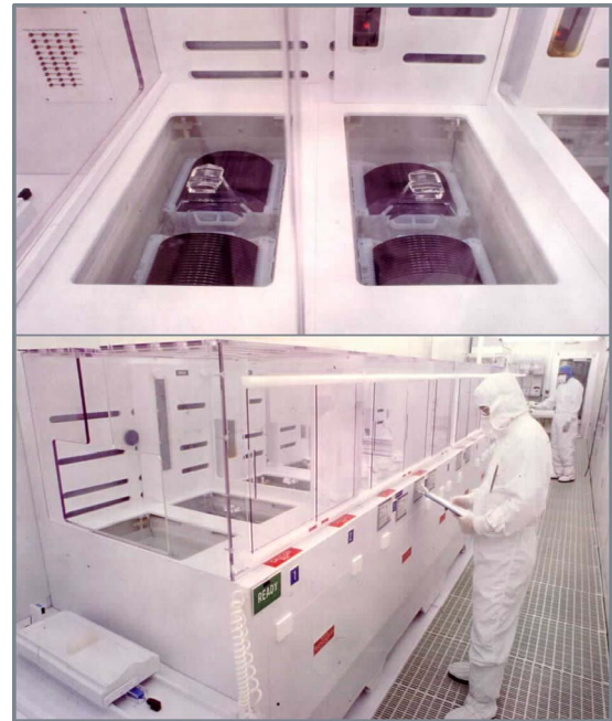
Fig. 10. A typical wet chemical bench for wafer cleaning.
