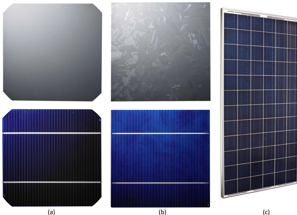
Fig. 17. Two types of silicon wafers for solar cells: (a) 156-mm monocrystalline solar wafer and cell; (b) 156-mm multicrystalline solar wafer and cell; and (c) 280-W solar cell module (from multicrystalline wafers).
