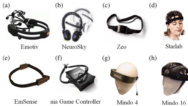
Fig. 3. Wearable EEG devices: (a) Emotiv, (b) NeuroSky, (c) Zeo, (d) StarLab, (e) EmSense, (f) nia Game Controller, (g) Mindo 4 with dry foam electrodes, and (h) Mindo 16 with dry spring-loaded probe sensors.
