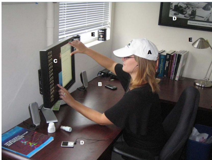
Fig. 2. BCIs based on pervasive technologies embedded in an office environment. A task-oriented BCI includes: (A) dry, wireless EEG sensors embedded into a baseball cap; (B) EEG signal collection and processing on portable smartphone, which also integrates with other devices in the environment; and is used to (C) improve human-computer interaction and work performance from online detection of cognitive and affective brain states, potentially including error-related signals, emotion, and time-on-task fatigue. The use of the task-oriented BCI avails opportunistic BCIs that (D) modify music selection and image in digital frame based on online detection of affective state; (E) alter lighting and office shades due to detection of oncoming migraine through EEG, and/or (C) cue the user to potential nonwork activities based on lack of sleep-based fatigue or stress. In addition, longer term data collection and analysis could result in diagnostics and recommendations for neural ailments.
