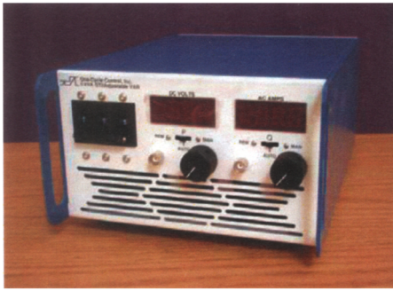
Figure 6. Grid-tied inverter with VAR generation (5kVA), courtesy of One-Cycle Control, Inc.
