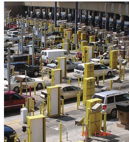
Fig. 12. A typical nuclear detection system incorporating radiation detection technology at a land border crossing. (Materials Today March 2008, Vol 11, No. 3)
