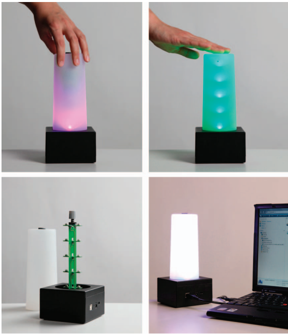
Fig. 3. Lantern is controlled by turning and pressing and uses light to indicate its status. It records the user actions which can be downloaded through a USB port.
