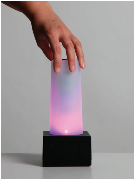
Fig. 1. Lantern is an interactive lamp that uses a simple visual grammar to display a piece of information.
