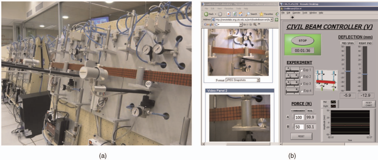
Fig. 1. UTS Remote Laboratory Facility ( http://remotelabs.eng.uts.edu.au ). (a) Physical equipment; (b) student interface to the Beam Deflection Experiment.
