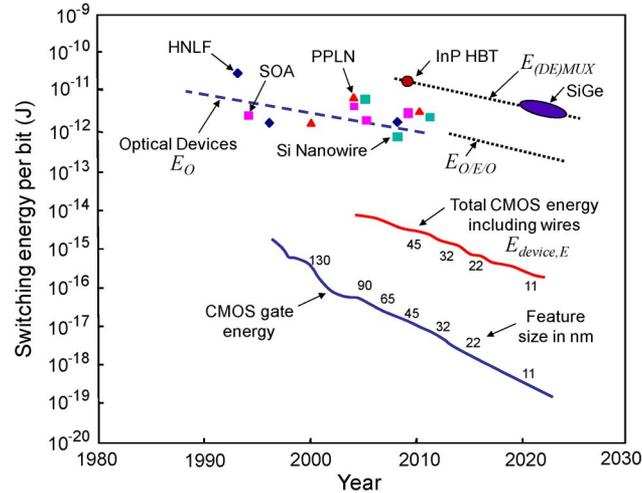
Fig. 4. Device energies per bit against time. The optical device energy per bit  $E_O$  is normalized to a reference clock frequency of  $f_{ref} = 100$  GHz. HNLF = highly nonlinear fiber, SOA = semiconductor optical amplifier, PPLN = periodically poled Lithium Niobate.
