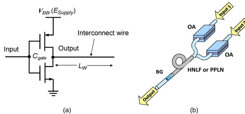
Fig. 2. (a) CMOS inverter circuit. (b) Schematic of a digital optical signal processing device providing switching by new frequency generation. PPLN = periodically polled Lithium Niobate. HNLF = highly nonlinear. OA = optical amplifier. BG = Bragg grating.
