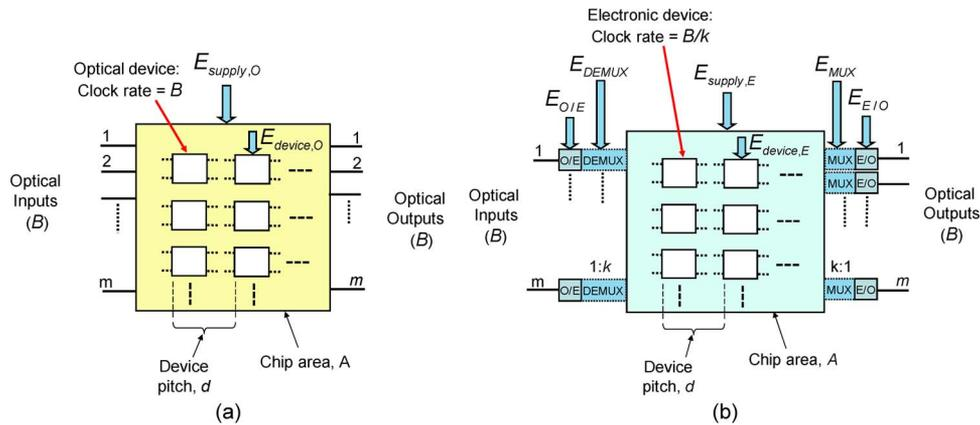
Fig. 1. (a) Optical signal processing circuit. (b) Electronic signal processing circuit.
