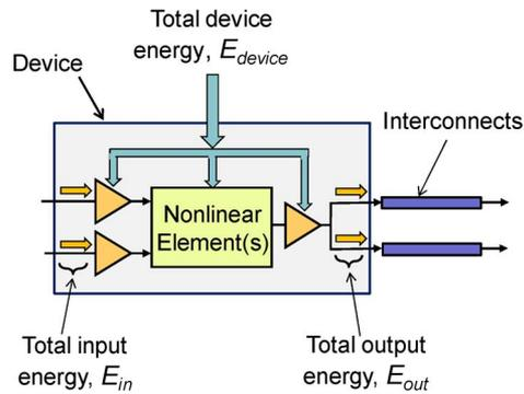
Fig. 3. Optical or electronic signal processing device with two input and two outputs. The device includes input and output amplifiers or buffers, and a nonlinear element.
