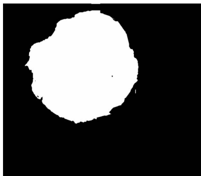
Fig. 4. Binary image used for area calculation obtained after thresholding Fig. 2(b).
