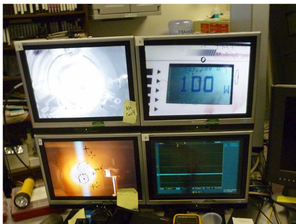
Fig. 1. Jefferson Lab high average power UV demo at 400 nm fundamental. (Upper left) Scatter from high reflectivity mirror. (Upper right) Average power. (Lower left) Light scatter from power probe. (Lower right) Time-dependent diagnostic.
