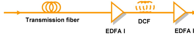
Fig. 1. Schematic of one span of fiber link consisting of a transmission fiber and a dispersion compensation fiber (DCF), which is sandwiched between two Erbium-doped-fiber-amplifiers (EDFA), i.e., EDFAs I and II.
