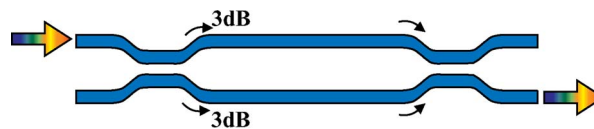
Fig. 3. Schematic of equivalent MZI.
