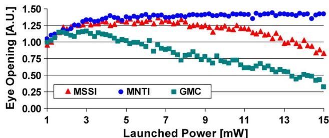
Fig. 3. Eye opening versus optical power launched into each span of the system, considering the NZDSF link. It can be seen that the eye opening obtained using the MNTI configuration is always larger than that given by the use of the other two approaches. All the curves reach the zero level for a sufficiently large launched power (not shown in the figure).
