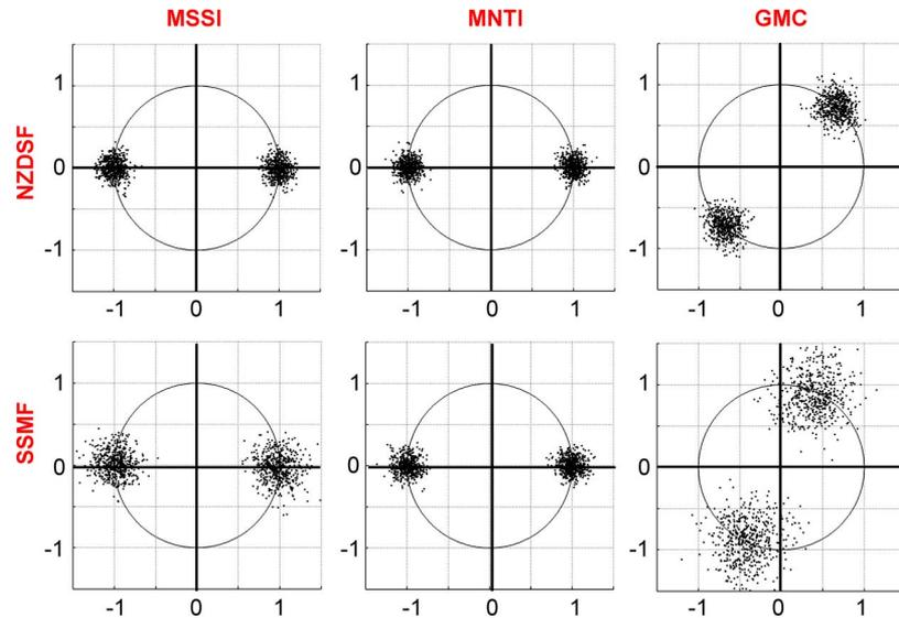
Fig. 2. Constellation diagrams obtained by the numerical simulation of the three different nonlinearity compensation techniques with different types of fiber. The constellation diagrams obtained without taking advantage of the OPC insertion are those reported in Fig. 1(h) (for NZDSF) and Fig. 1(l) (for SSMF).
