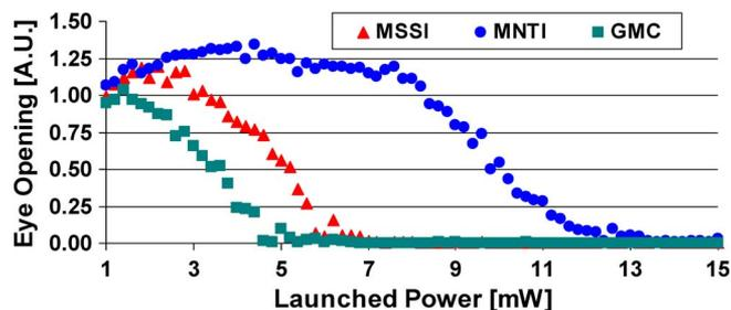
Fig. 4. Eye opening versus optical power launched into each span of the system, considering the SSMF link. It can be seen that the eye opening obtained using the MNTI configuration is always larger than that given by the use of the other two approaches. As the SSMF link is more sensitive to the fiber nonlinear effects, with respect to the NZ-DSF one, all the curves decrease more rapidly than those reported in the previous figure.
