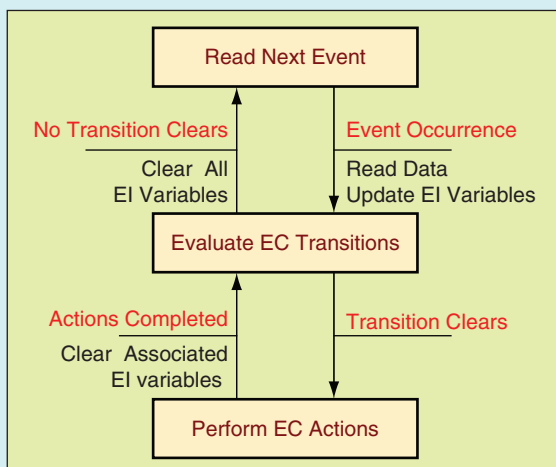
FIGURE 6—State machine of the active FB instance construct of IEC 61499.
