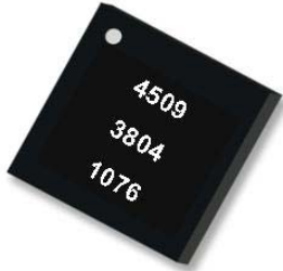
Fig. 2. 30-GHz PHEMT HPA in chip and packaged forms, TGA4509 and TGA4509SM
