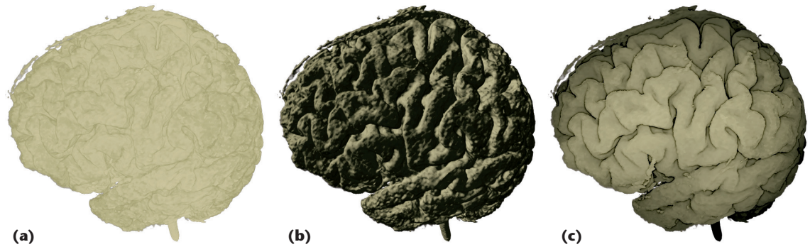
Figure 8. Two techniques for shading the brain (using the same transfer function). (a) No shading. (b) Gradient-based shading. (c) Depth darkening, in which dark means deep. Depth darkening depicts the brain structures more comprehensibly.
