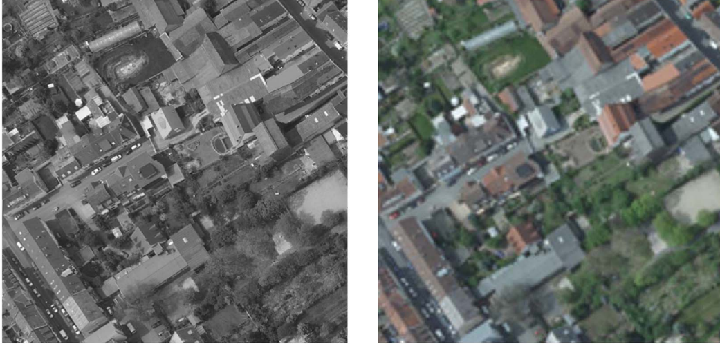
Fig. 3. Input images: (left) simulated HR pan image with a model error of 2.7%; (right) LR multispectral image obtained by downsampling the original HR multispectral image with a factor of 10.
