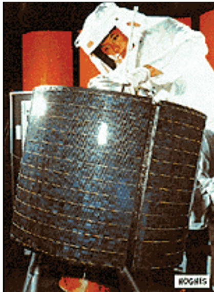
Figure 2. The Intelsat I (F-1), known in the world's press as "Early Bird." (Photo courtesy of the Comsat Legacy Project).
