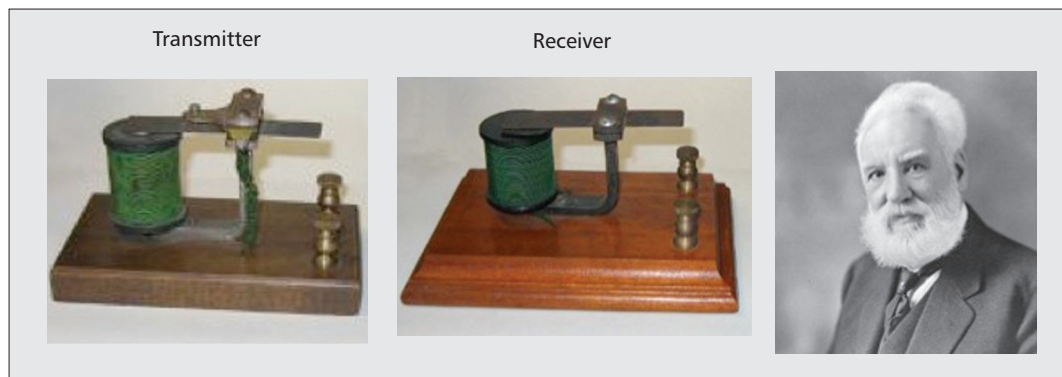
Figure 1. Bell's harmonic telegraph, using reeds responsive to different frequencies. Photos of replicas of the original equipment used with permission of Telecommunications Museum, LaSalle, Quebec, Canada.
