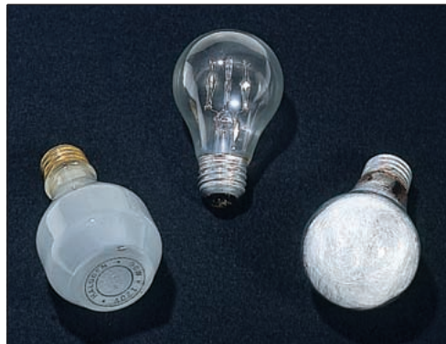
Fig. 5. Three experimental lamps show safety features intended to mitigate the risk of explosion. For example, in the Gemini lamp (center), note the small twin tubes paralleling the central glass stem—these low-pressure, 60-V halogen capsules would not explode. (SI neg. #2001-1914, by Richard Strauss. Left to right: GE AT-lamp with heavy glass envelope, circa 1990; “Gemini” lamp mock-up made by Elmer Fridrich, circa 1972; A-lamp with quartz-wool filling, also designed by Fridrich, circa 1972.)
