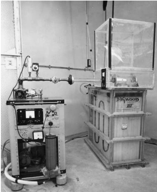
Fig. 2. 1.5-MV stacked stripline pulser “Dagwood.” The pulser is at the lower right. Above it is a gas-filled box containing the vacuum tube under test, evacuated by the pump on the left.
