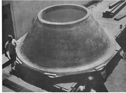
Fig. 21. 3-T 13-ft-diameter epoxy Brewster's angle vacuum interface cast by PI for the Pulserad 1590.
