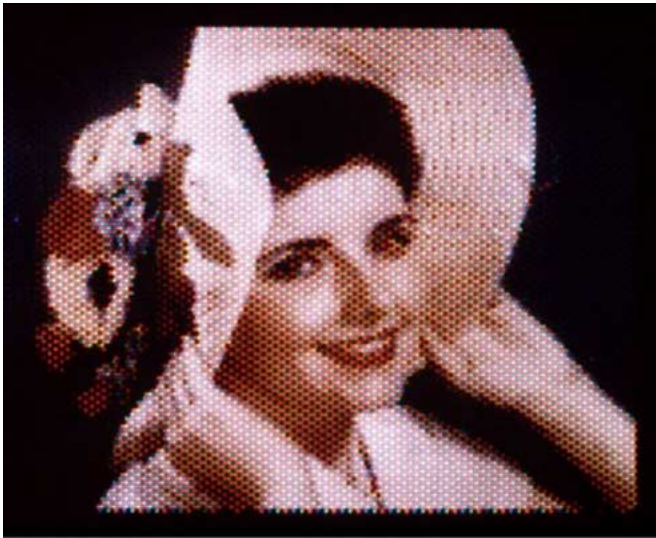
Fig. 15. Researchers at Hitachi achieved a record luminous efficacy of 1.5 lm/W with this dc plasma prototype in 1984 [27]. It used a new efficient discharge mode excited by very short high voltage pulses. This principle of very short pulsed discharges has also made ac plasma displays more efficient but in the ac case the discharge is short because of the action of the wall charge buildup which quenches the discharge.
