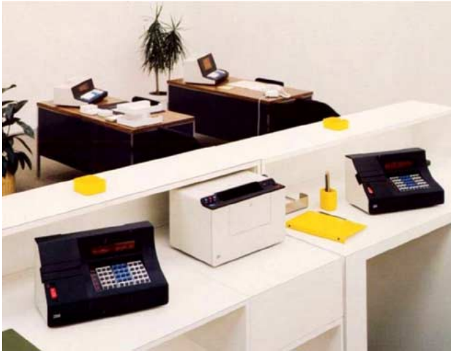
Fig. 11. IBM introduced a line of banking terminal products in 1973 that was the first plasma display product to use MgO as the cathode material. MgO was independently developed by IBM, Owens-Illinois, and Fujitsu in 1971. All of today's Plasma TVs use MgO cathodes.
