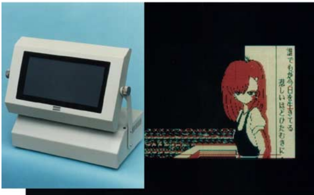
Fig. 18. Three-electrode color prototype developed by Fujitsu in 1984 [30]. It had three driven electrodes and one additional floating electrode. All electrodes were placed on the back plate, and only the phosphor on the front plate.
