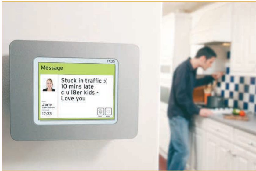
Figure 1. The Appliance Studio’s txTboard. The wall-mounted device displays SMS messages from family members or friends to its own phone number.
