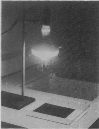
Fig. 5. Exposing Blue Poly film with sunlamp
