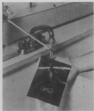
Fig. 6. Washing out Blue Poly after exposure
