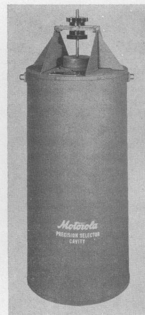
Fig. 4—Quarter-wave cavity selector used for base station control of intermodulation and desensitizing in the 160-Mc band.
