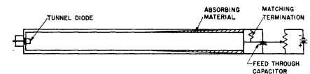
Fig. 2—Tunnel diode oscillator (output was taken from a probe at the diode end).
