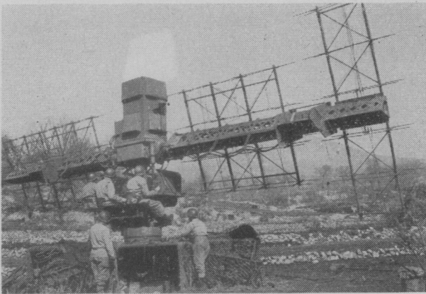
Fig. 23—Radio set SCR-268 with 5-man crew in operation on an Italian hillside. The three operators seated on the mount see indications of the airplane echo on cathode-ray oscilloscopes. One operator tracks the aircraft in azimuth (direction in degrees from north); another operator tracks in elevation (angular height); and the third measures the range.
