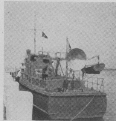
Fig. 5—Early experiments by Signal Corps Laboratories on 9-centimeter continuous-wave equipment located on Signal Corps boat. August, 1934.
