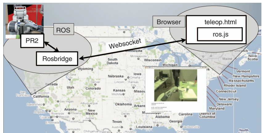
Figure 2. Connection diagram for a PR2 teleop application.
