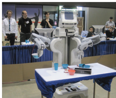
Figure 4. The PR2 robot being used by the world team in the 2012 ICRA Mobile Manipulation Challenge to clear a table.
