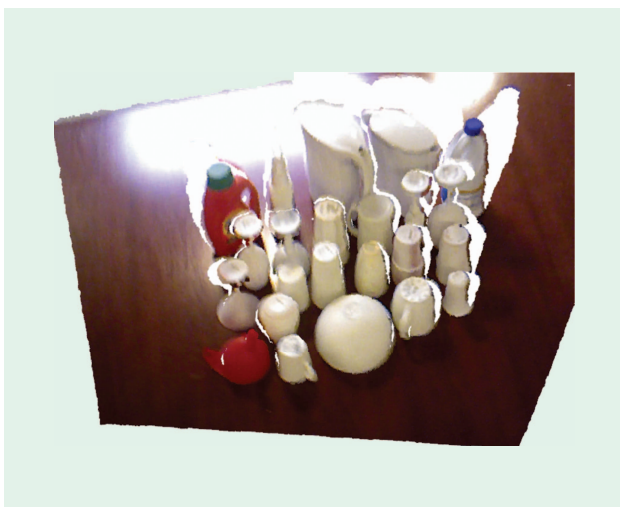
Figure 7. A subset of the objects used in the recognition experiments. The picture shows a screenshot of the point cloud obtained by the Kinect sensor with registered RGB information.
