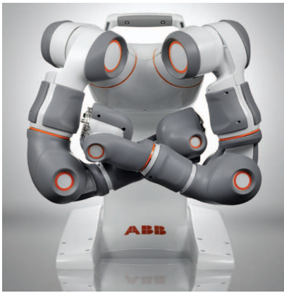
Figure 8. The ABB FRIDA concept is a 14-axis dual-arm robot designed for working alongside human workers in manufacturing environments. (Photo courtesy of ABB.)
