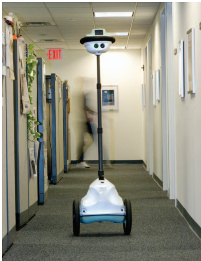
Figure 11. The QB telepresence robot by Anybots. (Photo courtesy of Randi Klett/ IEEE Spectrum .)
