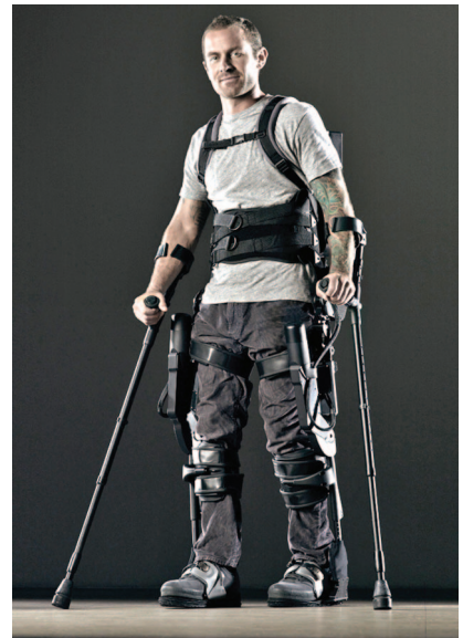
Figure 12. A test pilot tries the exoskeleton created by Ekso Bionics. (Photo courtesy of Ekso Bionics.)
