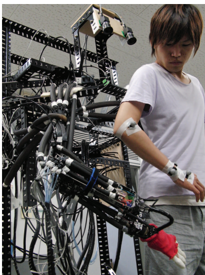
Figure 3. A robotic arm driven by McKibben pneumatic muscles and hand with flexible skin developed by Koh Hosoda and colleagues at Osaka University, Japan. (Photo courtesy of Koh Hosoda.)
