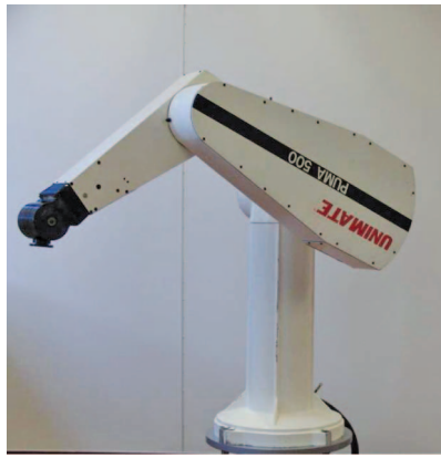
Figure 18. The classic Puma 560 arm is a chain of three rotatable bodies (excluding the end effector) attached to a rigid base. This yields a three-dimensional \mathcal{C} -space, which is handled by the standard planning algorithms. (Photo courtesy of the Technical University of Berlin.)
