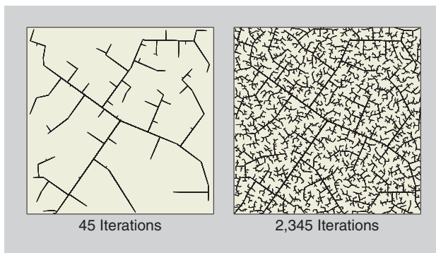
Figure 9. In the early iterations, the RRT quickly reaches the unexplored parts. However, the RRT is dense in the limit (with probability one), which means that it gets arbitrarily close to any point in the space.
