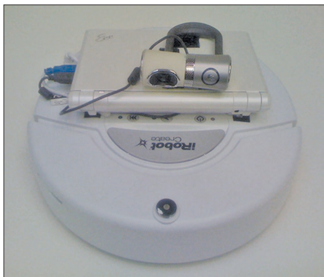
Figure 2. Brown University's small universal robotics vehicle, based on the iRobot Create, provides a versatile platform for ROS development.
