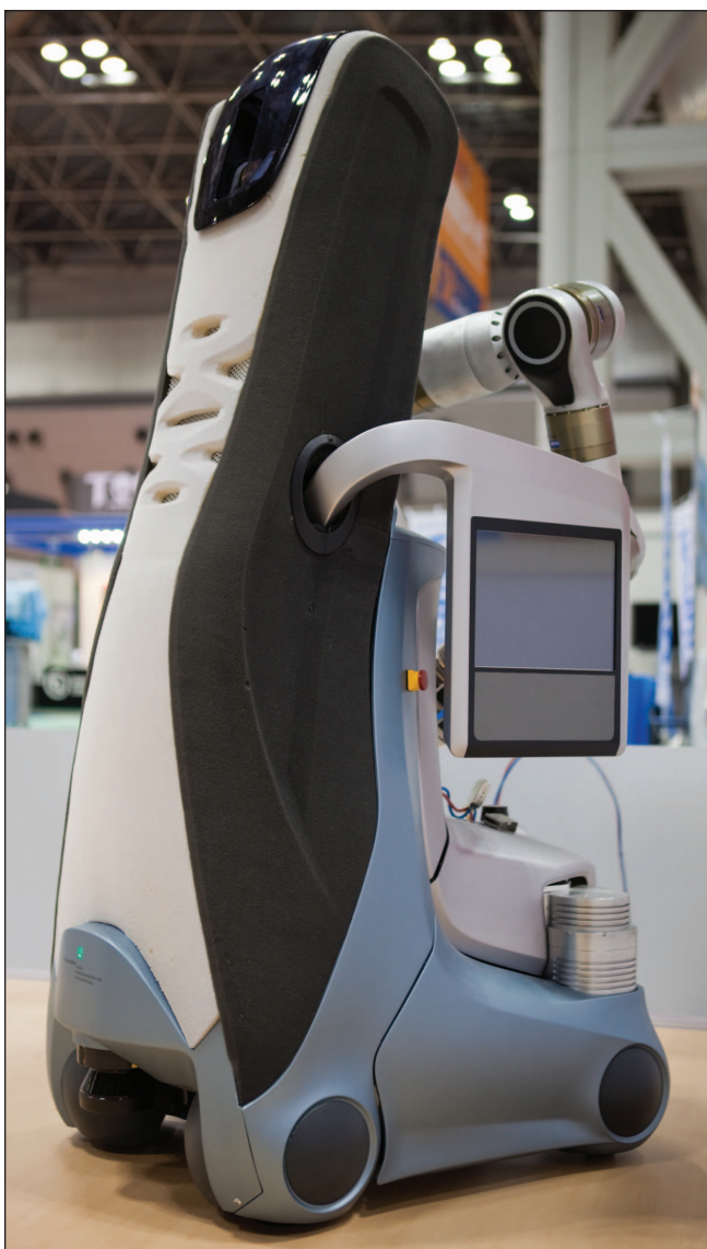
Figure 1. The Care-O-bot, first prototyped in 1998 at Fraunhofer IPA, is designed to be a mobile personal assistant.
